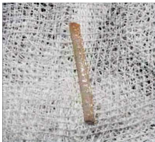
Fig. 3 3D printed polyactic acid (Cubex).
