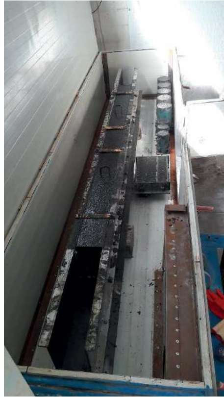
FIGURE 3: Casted beam specimen inside the oven.
