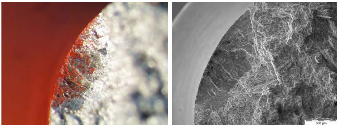
Figure 9 – Stereomicroscope and SEM images of fracture surface for specimen immersed in distilled water at 60 MPa for ~200 hrs.
