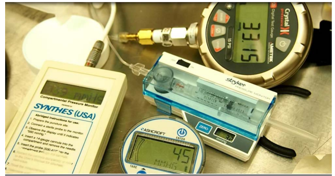
FIGURE 1. Image showing a screenshot of a recorded video indicating different pressure monitors in place during the experiment. The Stryker, Synthes, and MY01 were in the retroperitoneal space not in direct communication with the fluid or peritoneal cavity. The Ashcroft device was in line with the infuser providing reference for infusion pressure. The METEK device was in the peritoneal space communicating through a standing column of water.
