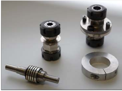
Fig. 1. Typical specimens for which the mass moment of inertia had to be determined by means of the presented pendulum set-ups.
