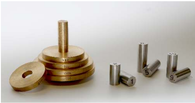
Fig. 7. Added mass-moment-of-inertia elements for the torsion pendulum (left) and for the physical pendulum (right).
