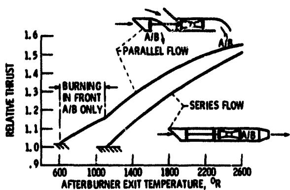
Figure 5. - Effect of afterburner temperature for parallel and series operating modes ( $\text{FPR}_{\text{DES}} = 1.4$ ).
