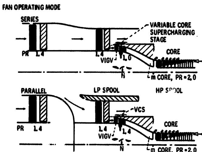
Figure 10. - Variable core supercharger.
