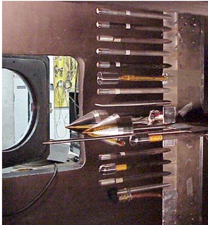
Figure 12: Survey Rake containing Pressure, Heat Transfer and Radiation Instrumentation.
