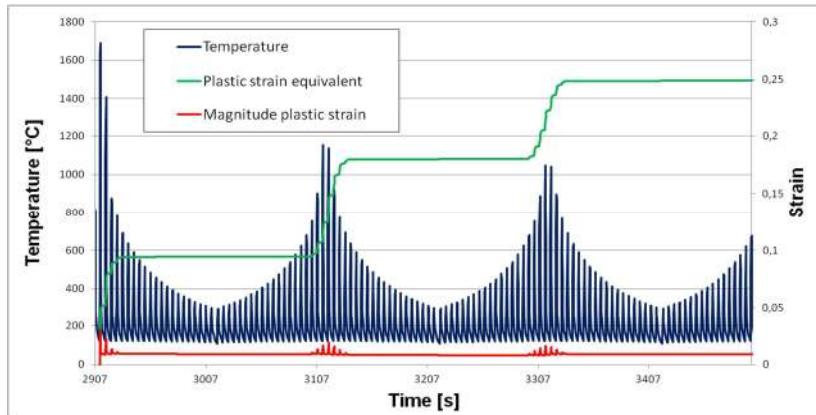
Fig. 6 Thermal and cumulated plastic strain variation in the element at the part centre
