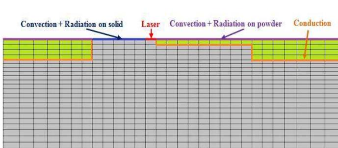
Fig. 2 Mesh and thermal boundary conditions
