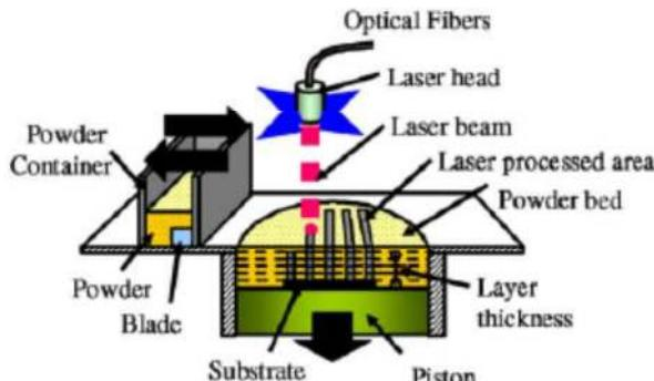
Fig. 1 Schematic illustration of SLM process according to [1]
