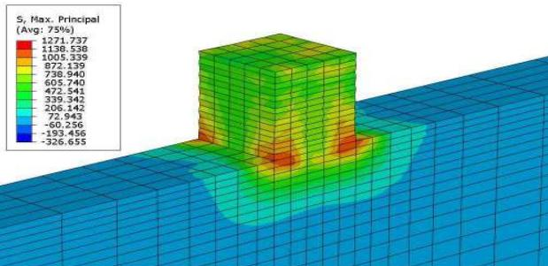
Fig. 8 Maximum principal stress in 3D model
