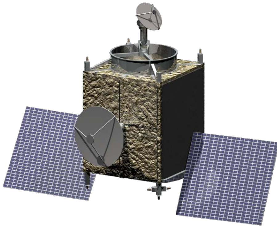
Figure B.3.—LRS deployed configuration, K/Ka band antenna face.
