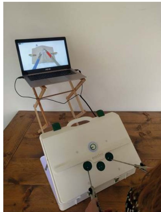
Fig. 1 The eoSim-augmented reality laparoscopic simulator interface
