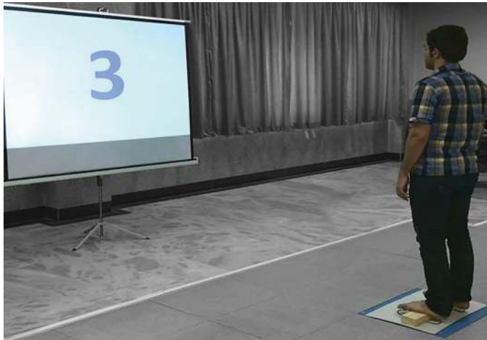
Figure 1. Experimental setup. Standing on a wooden block (9-cm wide in anteroposterior direction) placed on the force platform underneath the malleoli and facing the screen that displays digits printed in different colors.
