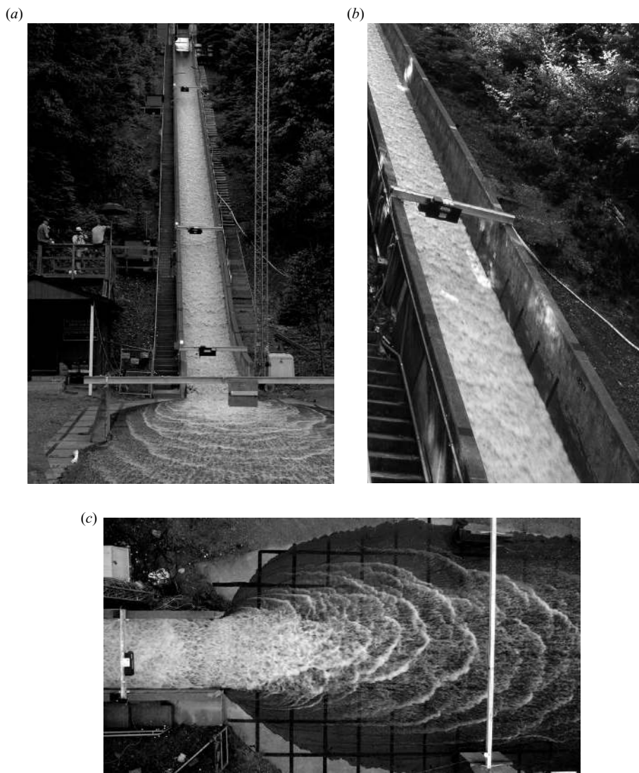
FIGURE 1. Photographs of a dam-break water flood descending the US Geological Survey debris-flow flume in the H. J. Andrews Experimental Forest, Oregon (Logan & Iverson 2007): front view ( a ) of a 6 \text{ m}^3 flood surge (the person in the foreground on the left-hand side provides an indication of scale), oblique view ( b ) from the right-bank platform of roll waves close to the depth sensor at a distance of 66 m from the gate and plan view ( c ) of water discharging at the end of the flume, showing many of the surface features of strong turbulence. The flume is a reinforced concrete channel 95 m long, 2 m wide and 1.2 m deep that slopes 31^\circ (60%).
