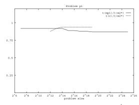
**Problem:** Compute  $\pi$  using the equation  $\pi = \int_0^1 \frac{4}{1+x^2}$ . **Approach:** Approximate the solution by computing  $\frac{1}{n}\sum_{i=0}^{n-1}\frac{4}{1+x_i^2}$  (rectangular rule), where *n* is the problem size parameter and  $x_i = (i + \frac{1}{2})/n$  is the midpoint of the
