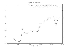
In the above diagram we compare the runtimes of two versions. The first version  $(t_{no-align-opt})$  has no ALIGNED WITH clause in the program text. The compiler produces code that detects dynamically at runtime whether adresses are local or not. In the second version  $(t_{align-opt})$ , alignment optimization in the compiler has produced ALIGNED WITH information. The code generator thus statically knows about locality. The diagram shows the arithmetic
