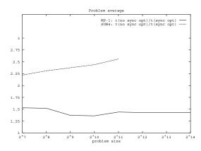
Synchronization barrier elimination improves runtime by over 40% on a MasPar and by over a factor of 2 on sequential workstations. Originally, the benchmark programs had 278 synchronization barriers which were reduced to 109 by applying the optimization technique.
