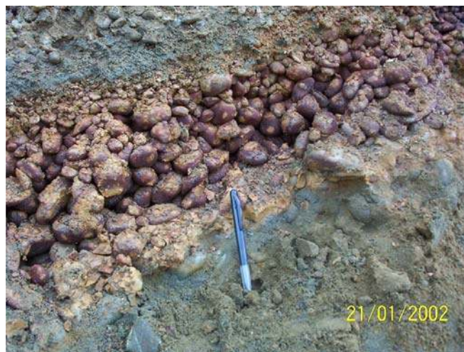
Fig. 2 Image of highly permeable channel material located within the Canterbury sandy gravels matrix; picture taken at a nearby site, from Davey (2006)
