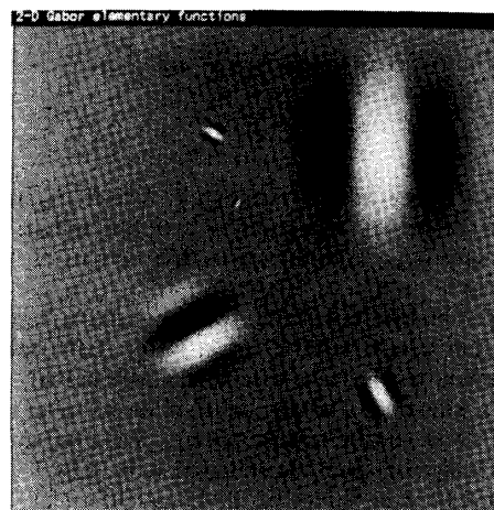
Fig. 6. Five examples of 2-D Gabor elementary functions displayed as luminance primitives. These biologically modeled "wavelets" can all be generated from a single complex member by dilations, rotations, and translations, as specified by (22).
