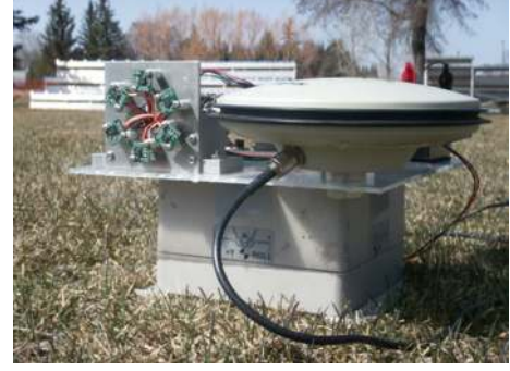
FIGURE 9: Test setup of the field data collection comprising the multi-magnetometer platform and the SPAN HG1700 GPS/INS system.
