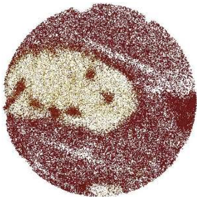
FIG. 1. Microstructure found by atom probe reconstruction of a \text{Cu}_{88}\text{Fe}_{12} sample, irradiated by 1.8 MeV Kr^+ ions at 350^\circ\text{C} to a dose of 3 \times 10^{16} ions/ \text{cm}^2 . The cross section of the 1-nm thick layer of atoms is about 50 nm in diameter. The Fe atoms (yellow) have been minimized to make the Cu atoms (red) inside the Fe precipitate more visible. Adapted from ref. 8.
