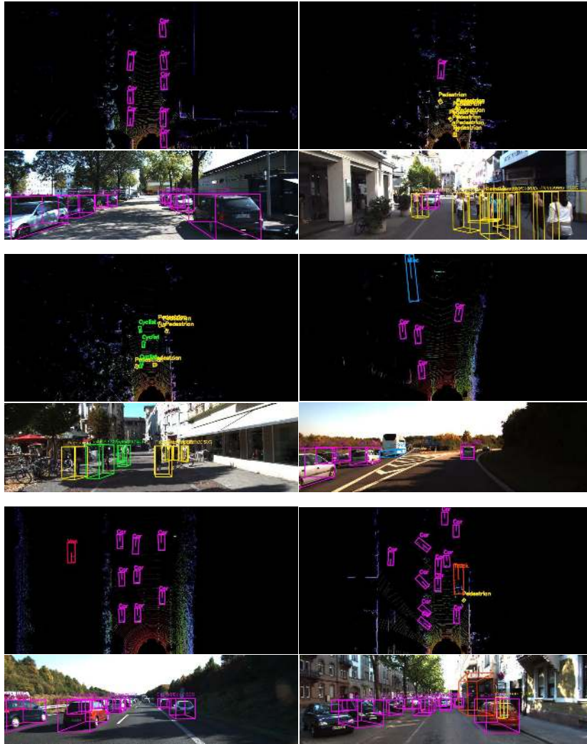
Fig. 6. Visualization of Complex-YOLO results. Note that predictions are exclusively based on birds-eye-view images generated from point clouds. The re-projection into camera space is for illustrative purposes only.
