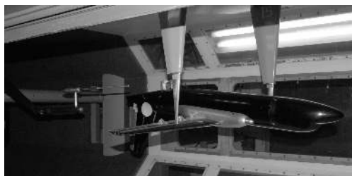
Figure 7.6: The F27 model as mounted belly-up in the wind tunnel. In the back the five-hole probe and traversing system can be seen.
