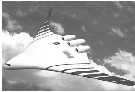
Figure 6.1: Artist impression of the Blended Wing Body concept as described by Liebeck[104]. [Image courtesy of NASA.]
