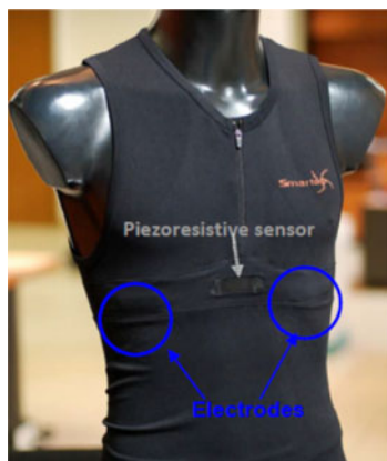
Fig. 2. Prototype of the PSYCHE wearable monitoring system showing a t-shirt with embedded textile sensors. From [17].
