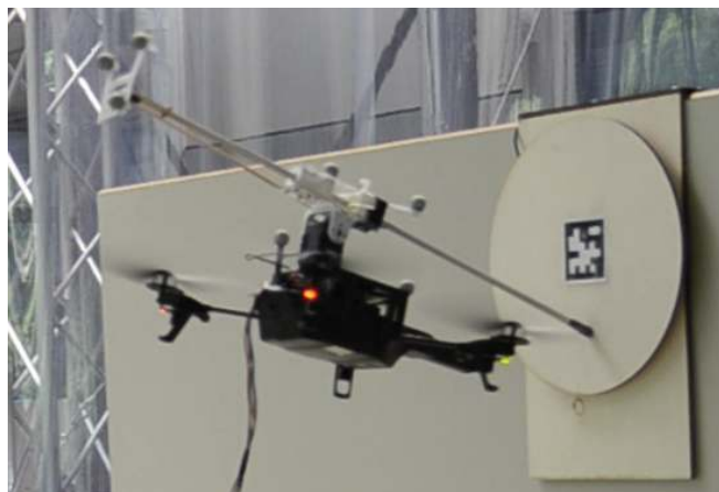
Fig. 1: Aerial manipulator achieving stable interaction after an impact with a vertical surface.
