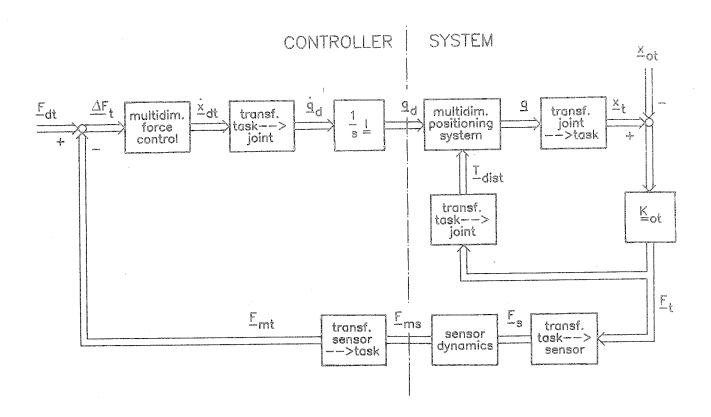
proximity sensing, and tracking directions in multidimensional compliant motion. Clearly, in case of noncontact sensors there is no external force which disturbs the position loop.
