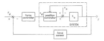
will be apt to exert controlled forces that make use of full actuator capability. Evidently, in such a case the contact force is no longer negligible. Therefore, we assume that the contact force can either be neglected or is compensated for by direct feedback of the actual measured force to the actuator drive torque.
