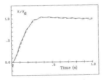
that h(s) is linear and second order (Eq. (6)) with  $\zeta_p = 0.75$ ,  $\omega_p = 11$  rad/s, and with negligible dead time (Fig. 9). In addition, a sufficiently strong decoupling exists between the operational space directions.
