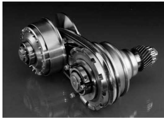
Figure 5.1: Van Doorne's pushbelt CVT
