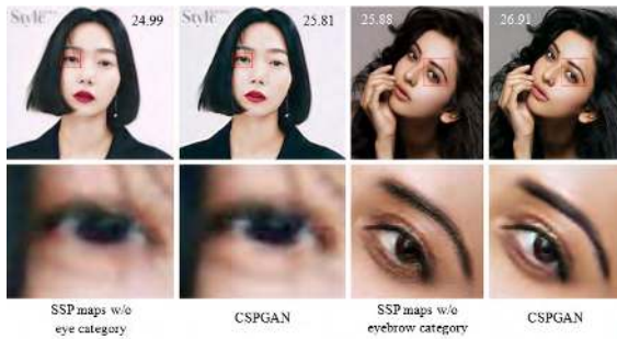
FIGURE 5. Effects of CSPGAN with or without certain facial component's category in the progress of reconstruction. When not labeling a semantic category, e.g. the 'eye' component, the generated facial images with magnified factor \times 8 will suffer blurry boundaries. The images of the upper row are integral reconstructed faces with their PSNR scores and images of the lower row are the details of the corresponding boxed patches.
