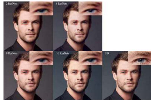
FIGURE 6. Effects of CSPGAN with different number of CSP Layers. The number of CSP layers has a strong influence on the reconstruction ability. Since they are embedded into the residual blocks, we prune the number of ResNets to test it. When n = 16 , the synthesized face appears most like the ground truth HR image. The upper right legends are the details of framed corresponding patches. (Zoom in for best view).
