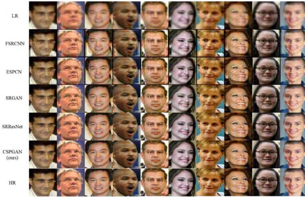
FIGURE 3. Comparison between different SR approaches with downsampling factor \times 4 in LFW dataset: FSRCNN [56], ESPCN [57], SRGAN [52], SRResNet [58], our proposed CSPGAN and the original HR image.
