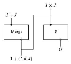
The type of Merge  $\boxplus p$  is  $(I + J) + (I \times J) \longrightarrow (1 + (I \times J)) + O$ . Thus the need for the  $xr_+$  output wrapping to fit the typing of the *partial feedback* combinator.
