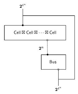
To specify Bus we adopt the following convention: the first cell in the  $\boxtimes$ -expression has coordinates  $\langle 1,1 \rangle$ , second is  $\langle 1,2 \rangle$  and so on until column n is reached; the next cell is then  $\langle 2,1 \rangle$ . Under this convention the output produced by cell  $\langle i,j \rangle$  is selected from the global output tuple as the  $j+(n\times(i-1))$ -projection, *i.e.*
