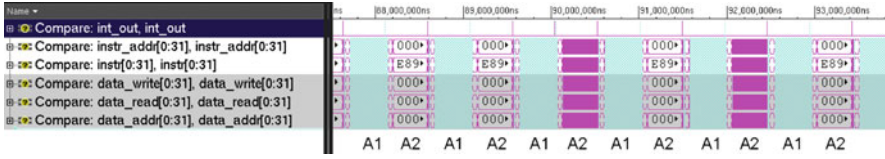
Fig. 2.10 MicroBlaze signal differences when A1 varies its behavior
