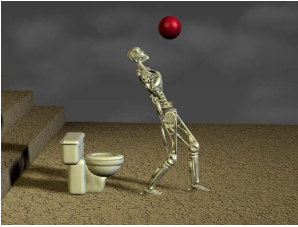
Figure 12: A still image from the terminator sequence. The dynamic terminator model has been knocked backward by the force of a collision to the head by the red ball. The terminator maintains balance by taking a protective step.
