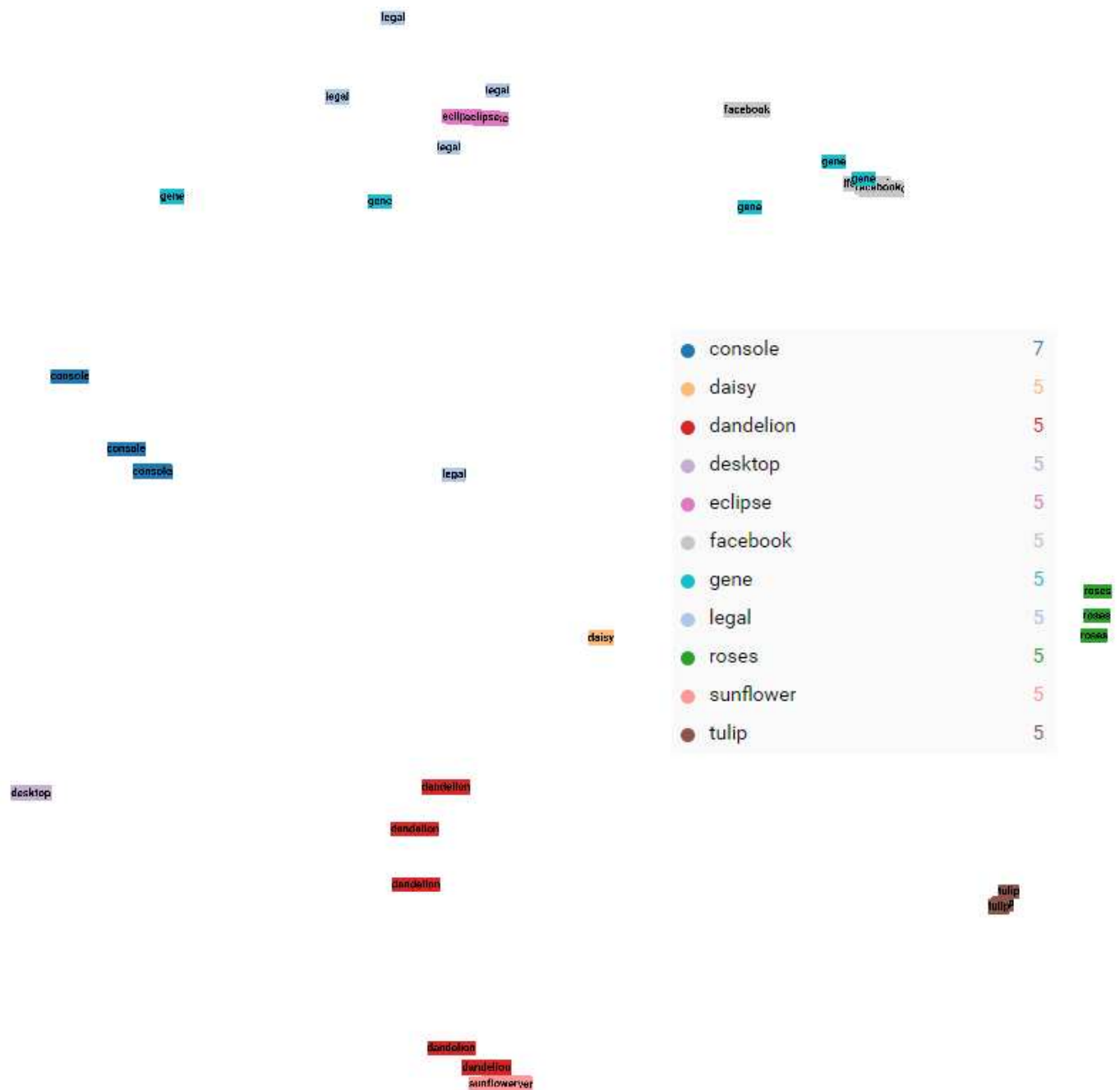
Figure 9.9: t-SNE representation of the feature vectors for images representing 11 contexts in 2D space. Each label in the figure represents an image. The text and color indicate the context the image belongs to. The clustering of the images by context indicates that the model learned to recognize and differentiate between the contexts. The default settings were used for perplexity (30). The model was executed for 2,936 iterations.
