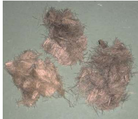
Fig. 2. Cut flax fiber used in the study
