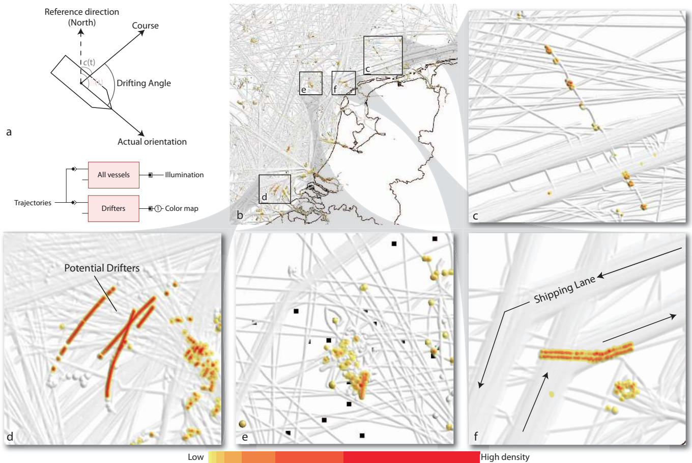
Fig. 8. Density maps of the area around the harbor of Rotterdam generated using a variable kernel based on (a) the velocity and (b) on traffic density. In (c) we use the density field of (b) as a illuminated height field and connect the area usage to the color component. In (a) more detail is visible in areas with slow moving or stationary vessels, such as inside the harbor and in anchorage areas. In (b) more detail is visible in dense areas such as the harbor mouth, the anchorage areas outside the harbor as well as the sea lanes. The block diagram for (a) is shown on the left, while the block diagram for (b) and (c) is shown on the right, with (b) with black and red links and (c) with black and green links.
