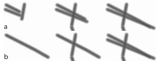
Fig. 6. Intermediate density fields for 1, 2, and 3 consecutive iterations over (a) time intervals and (b) individual objects.
