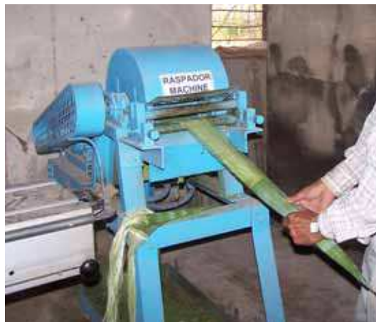
Fig. 3.2.1 Mechanical process of sisal fibre extraction using raspador machine
