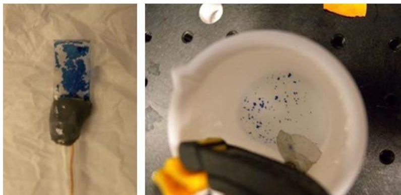
Figure 18. WO 3 electrodeposited on FTO (left) and electrolyte solution after multiple CVs (right).
