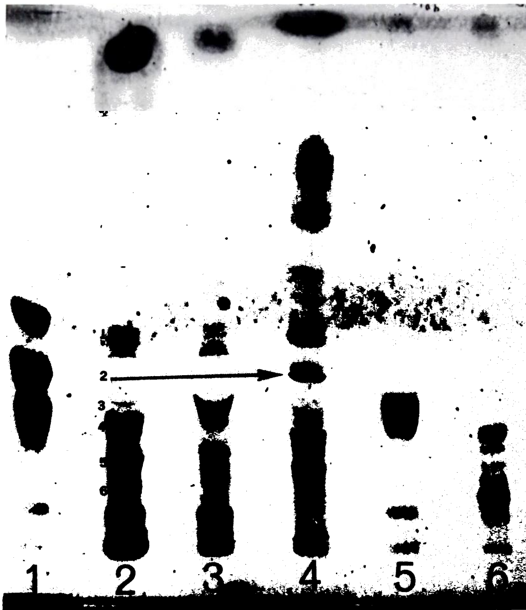
FIG. 2. Thin-layer chromatogram of ganglioside fractions from bovine testis tissue (4), seminal plasma (2), and sperm (3). The silica gel G plate was developed in chloroform-methanol-28 percent ammonia-water (60:35:7:3, by volume) and sprayed with resorcinol reagent. (1) Reference GM_3 , GM_2 and GM_1 in order of decreasing chromatographic mobility; (5) GD_3 ; and (6) GM_1 , GD_{1a} , and GD_{1b} , in order of decreasing chromatographic mobility).
