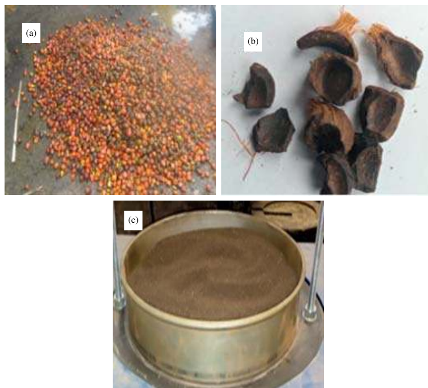
Fig. 1(a-c): (a) Palm kernel fruits, (b) Palm kernel shell and (c) Pulverised PKS
