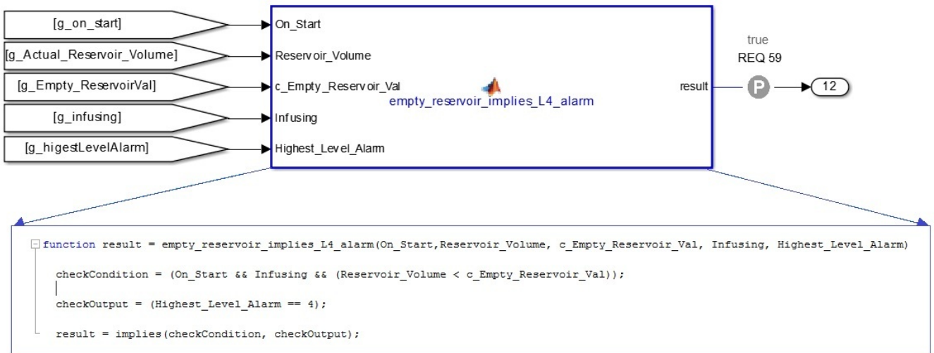
Figure 11: Alarm component property for Empty Reservoir check expressed in embedded MATLAB.
