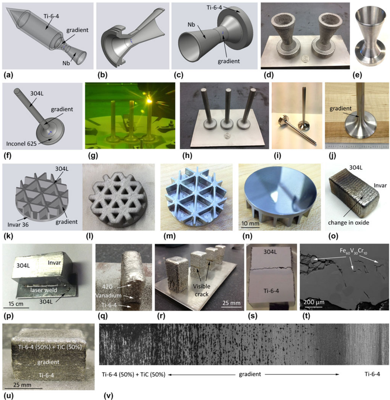
FIG. 7. Prototypes of gradient alloys fabricated using LD. (a–e) A Ti-6-4 to Nb rocket nozzle where the nozzle is fabricated from a high-temperature refractory metal, Nb, and the body of the rocket is fabricated from low-density Ti-6-4. (f–j) The fabrication of 304L to Inconel 625 valve stems where the valve is high-temperature Inconel 625 and the stem is 304L stainless steel. This part is typically made using a friction weld. (k–n) A 304L to Invar 36 gradient mirror with isogrid backing for increased stiffness. (o) A 304L to Invar 36 gradient alloy without any surface machining, showing the difference in oxide between the two alloys. (p) The alloy from (o) after surface machining and laser welding of a 304L plate, demonstrating weldability of the gradient alloy. (q) A successful gradient from Ti-6-4 to V, then from V to 420 stainless steel. (r) A similar gradient alloy to (q) but with a transition from Ti-6-4 to V, then from V to 304L, showing a crack. (s) After polishing, the crack at a specific composition is visible. (t) SEM micrograph showing that a brittle Fe–V–Cr phase has resulted in the cracking of the gradient alloy. (u) A Ti-6-4 to TiC gradient alloy. (v) Tiled micrographs from the gradient in (u) where the black phase is the TiC particles. This demonstrates the formation of a metal matrix composite using LD.
