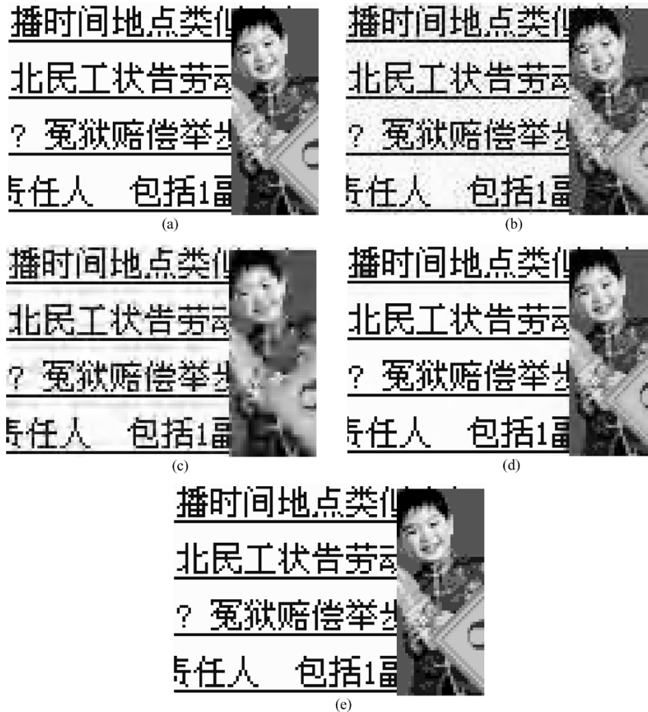
Fig. 13. Compression results of web2 . (a) A portion of the original image. (b) JPEG, 127 KB (11.3:1 compression). (c) JPEG-2000, 73 KB (19.4:1 compression). (d) DjVu, 84 KB (16.8:1 compression). (e) SPEC, 73 KB (19.4:1 compression).
