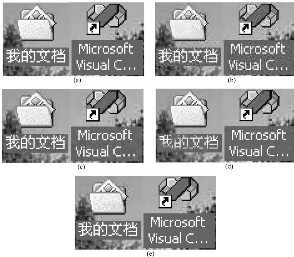
Fig. 15. Compression results of wall1 . (a) A portion of the original image. (b) JPEG, 90 KB (15.9:1 compression). (c) JPEG-2000, 112 KB (12.6:1 compression). (d) DjVu, 97 KB (14.5:1 compression). (e) SPEC, 112 KB (12.6:1 compression).
