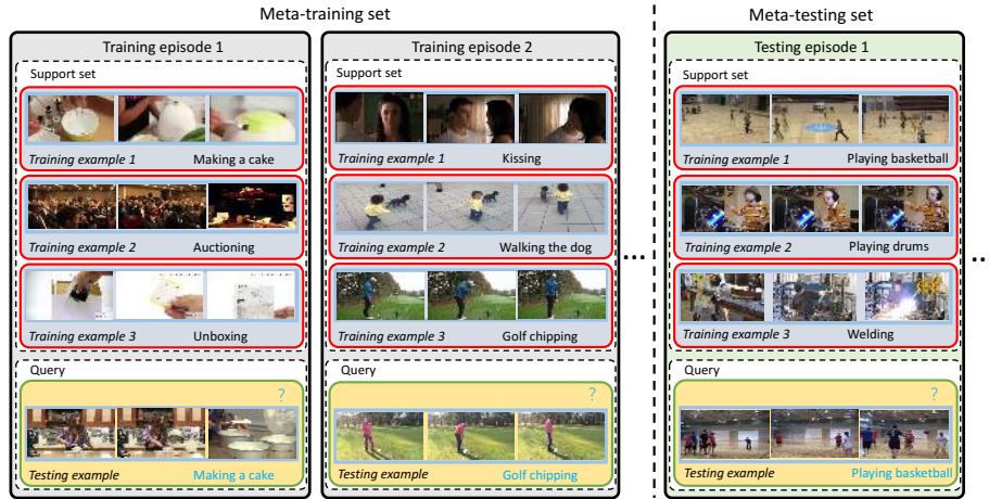
Fig. 1. The setting of the few-shot video classification. There are two non-overlapping datasets in this figure, i.e., meta-training and meta-testing. The meta-training set is for meta-learning and the meta-testing set is for evaluating the generalization performance on novel categories. The network is trained in an episodic way and each episode has a support set and a query example.
