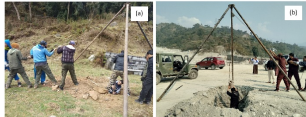
Figure 6. (a), (b) Standard penetration test at the sites
