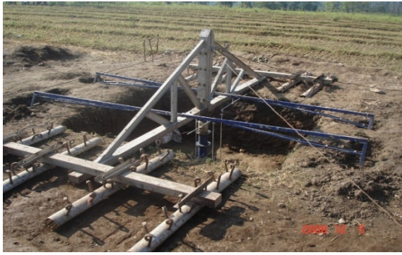
Figure 5. Overall set-up of the Plate Load Test (PLT)
