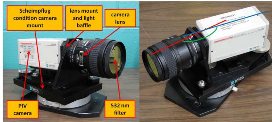
Figure 3.3 Stereo PIV camera assembly (left) depiction of offset between lens and sensor plane satisfying Scheimpflug condition (right).
