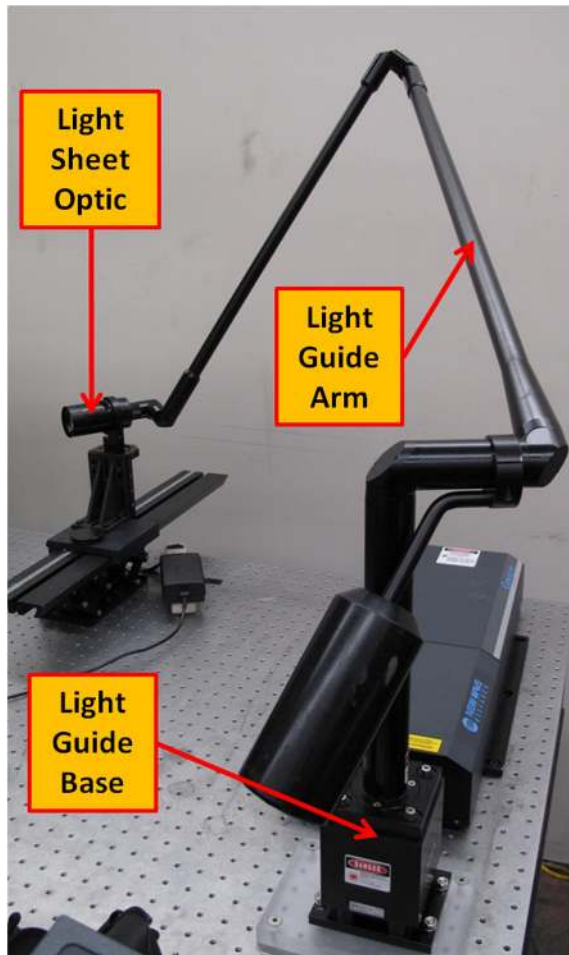
Figure 3.4 Dantec Dyanmic's light guide and sheet optic assembly.
