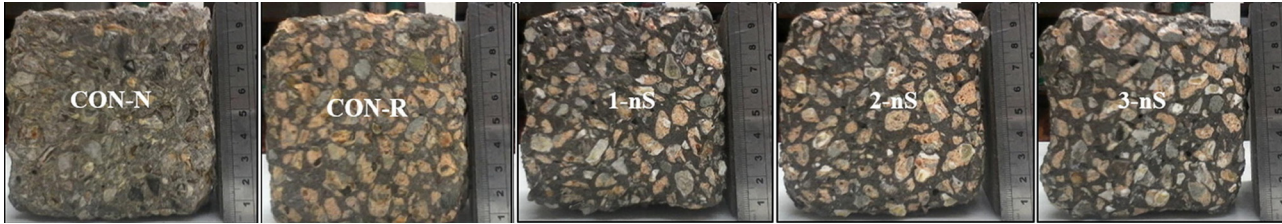
Figure 22: Geopolymer concrete specimens after 120 days immersion in 3% sulfuric acid [100].
