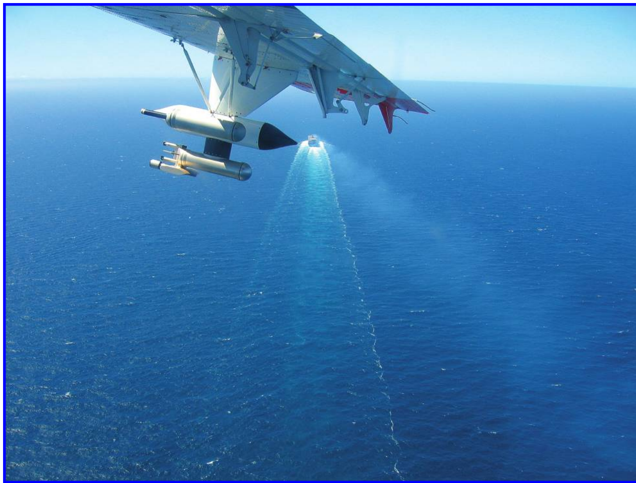
FIGURE 1. Photograph taken of the container ship from the cabin of the CIRPAS Twin Otter (the plane's wing tip is in the foreground) during the study. The exhaust plume is visible traveling with the mean wind at \sim 10^\circ angle to the heading of the ship, which can be inferred by the visible wake.
