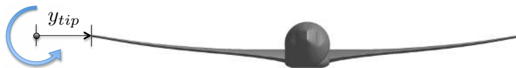
Figure 17. Positioning defined from center of nearest vortex from upstream aircraft to wingtip of trailing aircraft.
