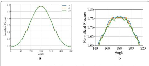
**Fig. 12** Comparison: Moving cylinder for different mesh refinement levels (L) over the angle. **a** Surface pressure of the cylinder geometry over the angle for different mesh resolutions. **b** Zoom-in of the stagnation area (maxima)
