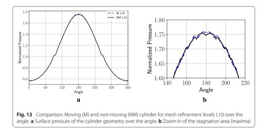
behavior for both cases is very close and in agreement with each other. We can observe a slight shift in the stagnation point between both solutions (cf. Fig. 13b), which is again due to the movement of the cylinder and the different representation in each time step. However, apart from that, both curves show the same behavior in pressure and are in very good agreement.
