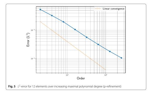
shift of the reflected wave gets diminished with increasing orders. With sufficiently large degrees of freedom, the wave shows an excellent agreement with the reference solution. The error convergence is done in reference to this solution.
