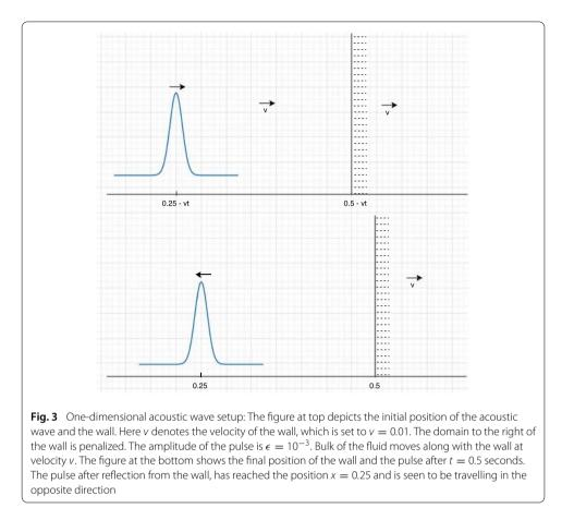
should have the same shape and size, only with opposite velocity. After the simulation time of t = 0.5, with linear acoustic wave transport and a speed of sound of 1, the position of the pulse will again be at a distance of d = 0.25 away from the position of the wall at that time. During this duration, the wall travels a distance of vt to the right, reaching the point x = 0.5. Therefore, the final position of the pulse has its center x = 0.25 after the time interval t.
