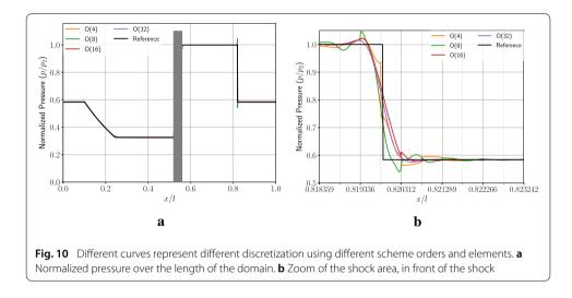
apply a smoothing filter that addresses Gibbs oscillations close to the shock [28]. As in the previous Sect. Reflected shock wave with the reflected shock, we consider discretizations with different scheme orders (O) but with the same overall number of degrees of freedom. We use spatial schemes of order O(4), O(8), O(16) and O(32) with element counts (n) of n2048, n1024, n512 and n256, respectively. Thus, the domain is resolved by 8192 degrees of freedom in each case.
