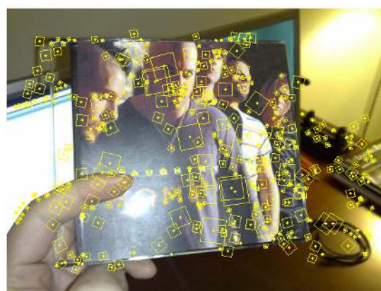
Figure 1. Typical query image with m features. Note that the features in the image can be transmitted in any order. As a result, by clever ordering of the feature set, one can reduce the query size by \log_2(m!) bits.
