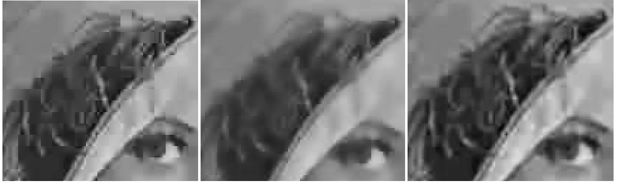
Figure 8. A region from our experiment with the Lena image is displayed. Image size is 128 \times 128 ; and the bit-rate for the compressed image is 0.18. From left to right: (a) The standard bilateral filter with \sigma_r = 20 , \sigma_d = 3 ; (b) The standard bilateral filter with \sigma_r = 50 , \sigma_d = 3 ; (c) The adaptive bilateral filter with \sigma_{r,min} = 20 , \sigma_{d,min} = 3 , k_0 = 1.0 , k_1 = 10.0 .
