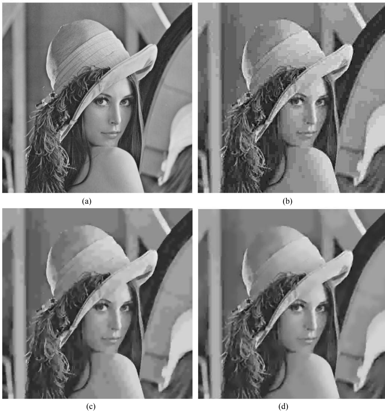
Figure 10. The experiment with the Lena image is displayed. Image size is 512 \times 512 ; and the bit-rate for the compressed image is 0.18. (a) Original image; (b) Input compressed image; (c) The standard bilateral filter with \sigma_r = 20 , \sigma_d = 3 ; (d) The adaptive bilateral filter with \sigma_{r,min} = 20 , \sigma_{d,min} = 3 , k_0 = 1.0 , k_1 = 10.0 .
