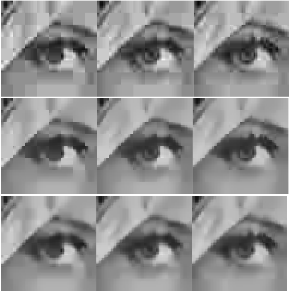
Figure 9. A region from our experiment with the Lena image is displayed. Image size is 64 \times 64 ; The first row shows the compressed image, the second row shows the original Bilateral filter, and the third row presents the proposed method. From left to right the bit-rate is 0.18, 0.22, 0.24. k_0 = 1.2 , k_1 = 10.0 , \sigma_{r,min} = 20 , \sigma_{d,min} = 1.5 , \sigma_r = 20 , \sigma_d = 3 .
