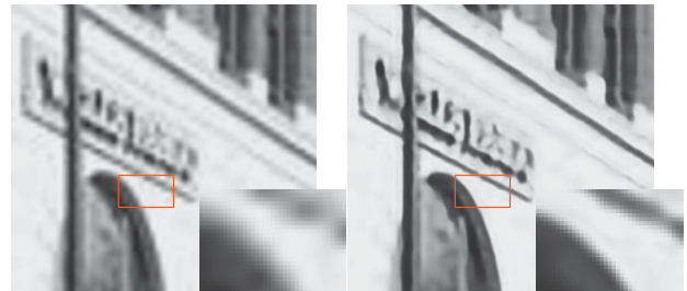
(b) Left: the Twitter-compressed image, which is first re-scaled to a small image and then compressed on the server-side. Right: the restored image by the proposed deep model (AR-CNN)
