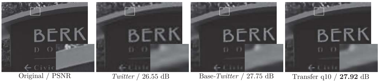
Figure 12. Restoration results of AR-CNN on Twitter compressed images. The original image (8MP version) is too large for display and only part of the image is shown for better visualization.
