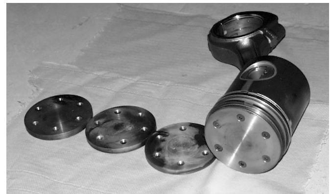
Figure 2. The piston, with the 15:1 compression ratio crown assembled. To the left of the piston is shown the crowns for 17:1, 20:1 and 21:1 compression ratios.
