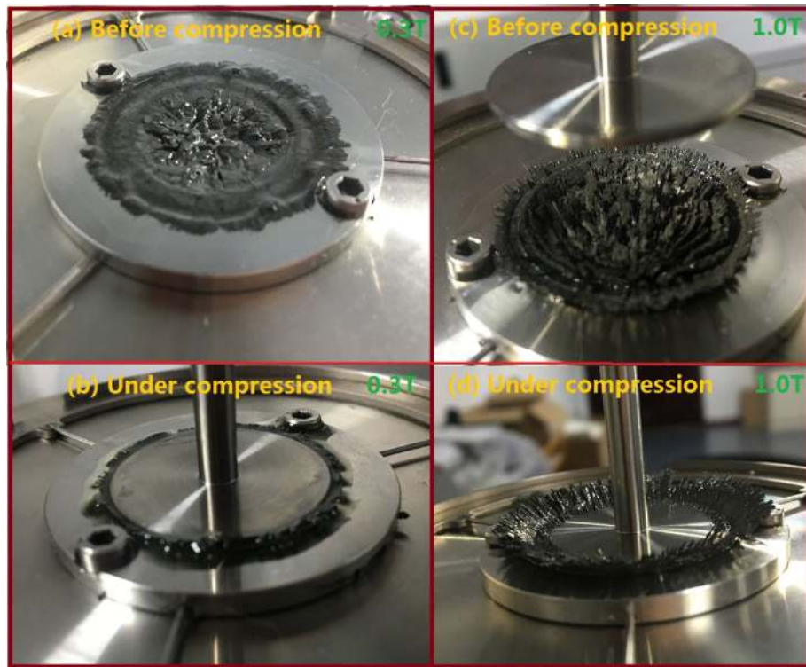
Figure 4. Photos of the MR fluids in the experiment. (a) Before compression with B_0 = 0.3 T; (b) under compression with B_0 = 0.3 T and \epsilon = 0.7 ; (c) before compression with B_0 = 1.0 T; (d) under compression with B_0 = 1.0 T and \epsilon = 0.7 .
