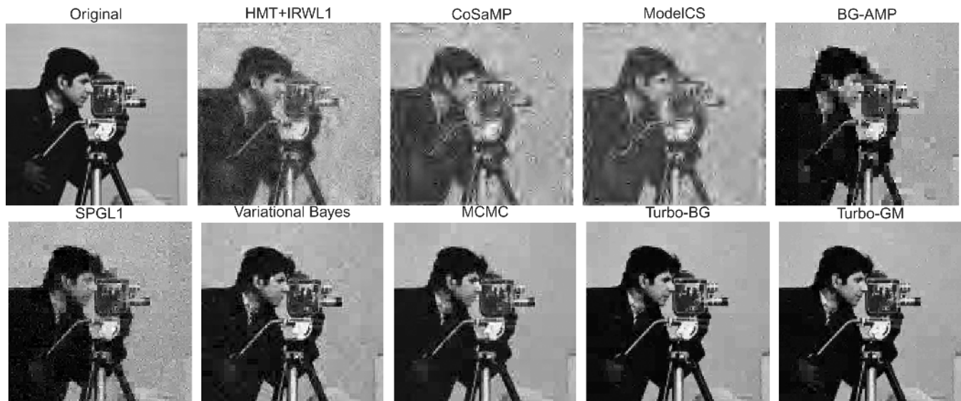
Fig. 4. Reconstruction from M = 5000 observations of a 128 \times 128 (i.e., N = 16384 ) section of the cameraman image using i.i.d. Gaussian \Phi .
